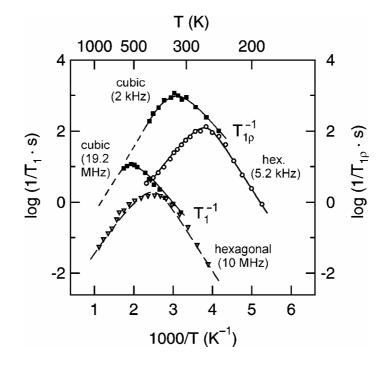
**Fig. 4:** Temperature dependence of laboratory and rotating frame spin-lattice relaxation rates of cubic  $Li_{0.6}TiS_2$  and hexagonal  $Li_{0.7}TiS_2$ . Rotating frame data were recorded at about 2 kHz for cubic  $Li_{0.6}TiS_2$  and at 5.2 kHz in the case of hexagonal  $Li_{0.7}TiS_2$ . The corresponding data in the laboratory frame were measured at 19.2 MHz (cubic) and 10 MHz (hexagonal), respectively. Data of the hexagonal modification were taken from Ref. [11].
