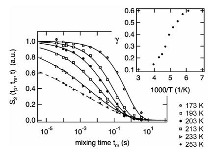
**Fig. 5:** <sup>7</sup>Li spin-alignment echoes of cubic  $\text{Li}_{0.6}\text{TiS}_2$  as a function of mixing time. Data were recorded for fixed evolution time  $t_p = 12 \ \mu\text{s}$  and at 155 MHz. Between 173 and 253 K the decay curves follow stretched exponentials (fit curves shown). The inset displays the stretching exponents *vs* reciprocal temperature.
