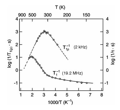
**Fig. 3:** Laboratory and rotating frame spin-lattice relaxation rates of cubic  $\text{Li}_x \text{TiS}_2$  vs reciprocal temperature. Relaxation rates were recorded at a resonance frequency of 19.2 MHz and at a locking frequency of 2 kHz. The Larmor frequency of the rotating frame experiments was 77.8 MHz. Rotating frame data were taken from Refs. [12,24].
