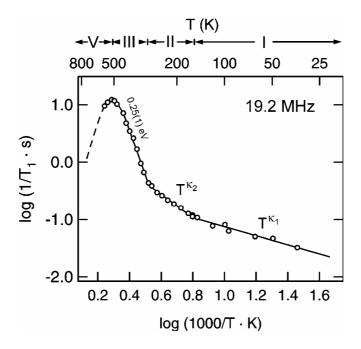
**Fig. 2:** Temperature dependence of the laboratory frame spin-lattice relaxation rate  $1/T_1$  of cubic Li<sub>x</sub>TiS<sub>2</sub> with x = 0.6. In ranges I and II the rate follows a weaker-than-activated temperature dependency which can be expressed by two power laws with the exponents  $\kappa_1$  and  $\kappa_2$ . The flank of the diffusion induced rate maximum shows up above 315 K. Data were taken from Refs. [12,24].
