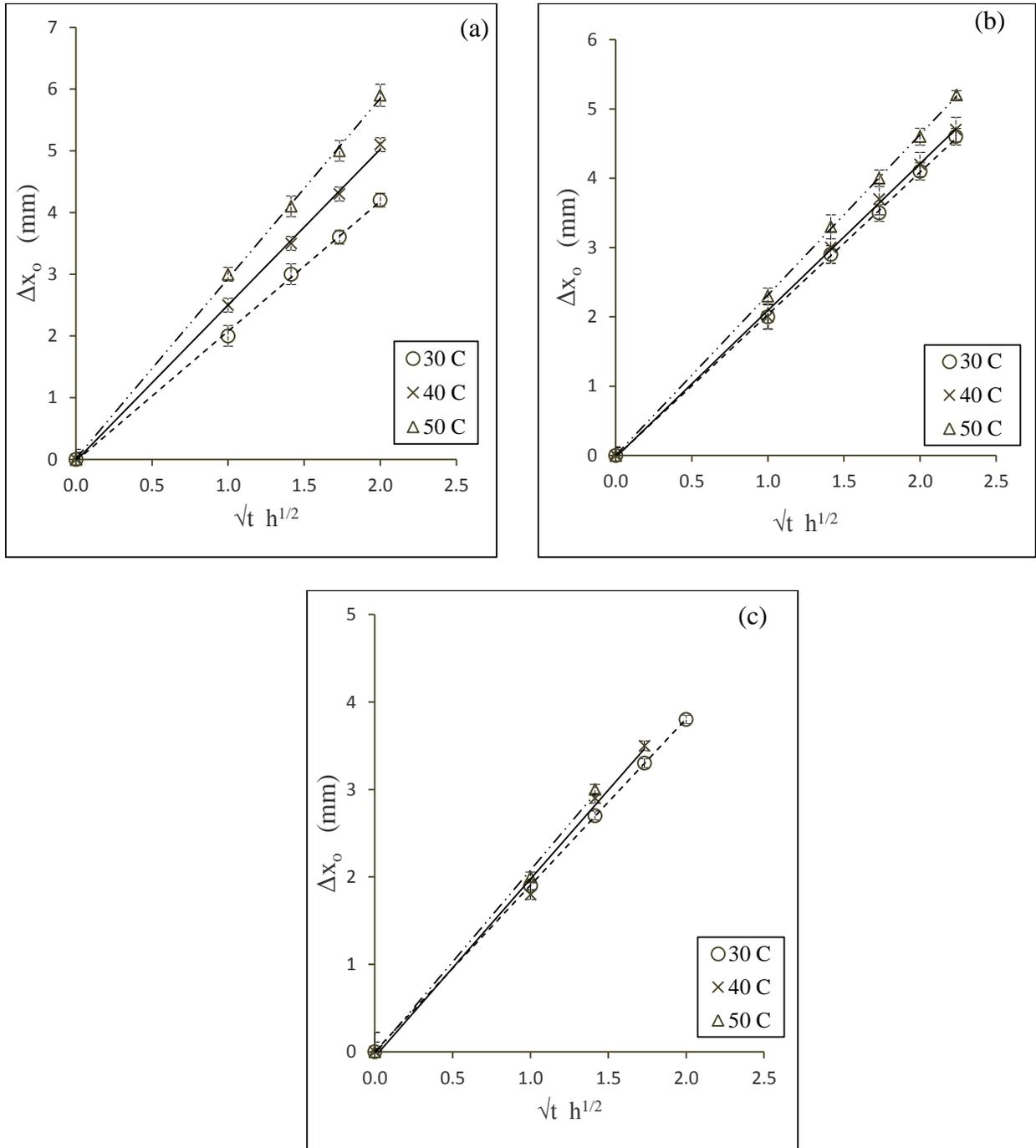
**Fig. 4:** (a) Experimental data fitted to theory in form of movement of the interface versus  $\sqrt{t}$  are shown (a) at 30°, 40° and 50 °C for hexane, (b) at 30°, 40° and 50 °C for heptane and (c) 30°, 40° and 50 °C for toluene.
