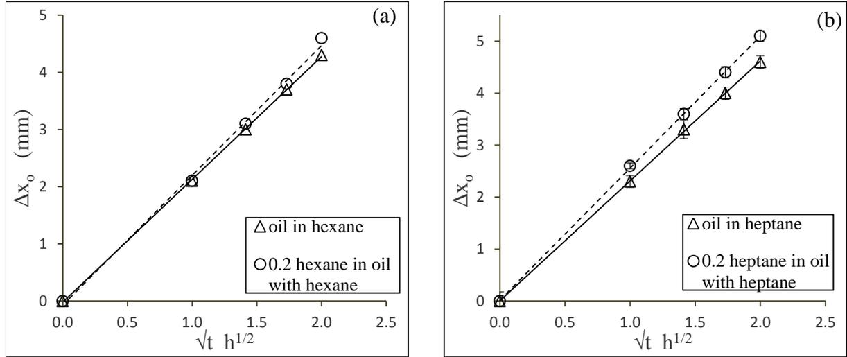
**Fig. 5:** Experimental data fitted to theory in form of movement of the interface in dissolution of oil for (a) pure oil in hexane and oil with 0.2 volume fraction hexane dissolving in pure hexane, and (b) pure oil in heptane and oil with 0.2 volume fraction heptane dissolving in pure heptane, both at 50 °C.
