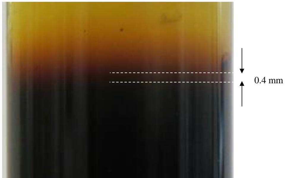
**Fig. 2:** (a) Interface between heavy oil and solvent, hexane, from 0 to 4 hours at 30 °C. Solvent interface height decreases with time. The sample was allowed to rest for 48 hours at room temperature and diluted oil was poured out to reveal asphaltene precipitation on the sides of the test tube. (b) Enlarged portion from a heavy oil-hexane sample at 4 hours showing the interfacial region. Interface is not of zero thickness, but about 0.4 mm thick.
