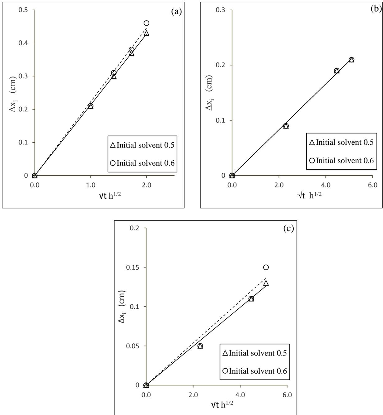
**Fig. 6:** Experimental data fitted to theory for desorption at 50 °C of (a) oil with 0.5 and 0.6 volume fraction hexane (b) oil with 0.5 and 0.6 volume fraction heptane and (c) oil with 0.5 and 0.6 volume fraction toluene.
