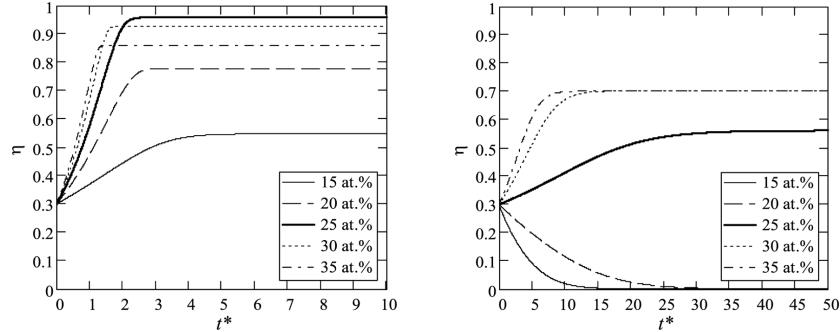
Fig. 1: The reduced-time dependences of  $L1_2$ - and  $D0_{19}$ -type LRO parameters for different atomic fractions of alloying component at the reduced temperatures  $T^* = 0.12$  (left) and  $T^* = 0.20$  (right).
