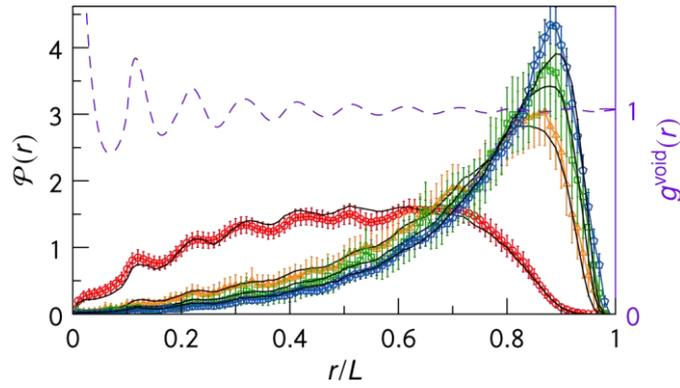
Figure 8: The renormalized persistence length  $\ell_p^*$  can approximately account for the disorder-modulated radial distribution function  $\mathcal{P}(r)$  (here shown for  $\ell_p = 2D$  (red),  $\ell_p = 6D$  (orange),  $\ell_p = 8D$  (green),  $\ell_p = 10D$  (blue)), if the renormalized WLC result is multiplied by the void space distribution function  $g^{\text{void}}$ . Reproduced from Ref. [9].
