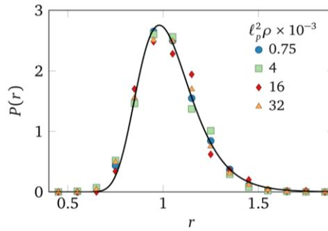
Figure 9: Tube size distribution obtained from the binary collision approximation (solid line), Eq. (18), compared to hybrid Monte Carlo / Brownian dynamics simulations (symbols) by Ramanathan and Morse [24] for a concentration range ( $\rho$  is the polymer length per volume) comparable to that realized in typical experimental systems. In the simulations, the tube size is measured after a characteristic time interval at which the growth of the polymers' transverse MSD slows down.
