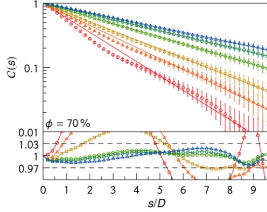
Figure 6: The numerically determined tangent correlations decay exponentially in the limit  $\ell_p/D \rightarrow \infty$  (here shown for  $\ell_p/D = 2, 3, 4, 6, 8, 10$  and a background filling fraction of 70 %), and decay more quickly for higher disorder filling fractions  $\phi$ . The relative deviations of our exponential fits to the data are shown in the lower panel. Above  $\ell_p = 6D$ , these deviations nowhere exceed  $\approx 3\%$ . Reproduced from Ref. [9].
