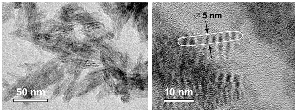
(HR)-TEM images of TiO<sub>2</sub> nanorods investigated electrochemically. The rods show lengths in the order of 20 to 30 nm; the mean diameter is approximately 5 nm.
