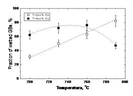
Figure 1: (left) The microstructure of Ti–4 wt.% Co alloy annealed at  $760^{\circ}$ C, 816 h. The  $\alpha$ -Ti phase appears light, the  $\beta$ -(Ti, Co) phase appears dark. (right) Temperature dependence of the fraction of completely wetted GBs for alloys: Ti-2wt.% Co and Ti-4wt.% Co.
