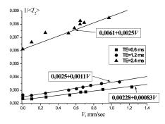
Figure 1: The dependence of the average relaxation rate  $1/\langle T_2 \rangle$  on fluid flow velocity (Berea core).
