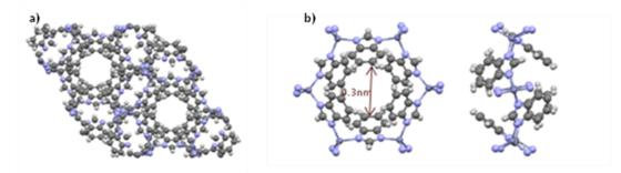
Figure 1: ZIF-7 unit cell (a). The main six-member window of ZIF-7 (b); Top view (left), side view (right).
