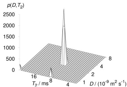
Fig. 2: inverse Laplace transformation of Fig. 1 with single peak at  $T_2 = 8\text{ms}$  and  $D = 2.3 \times 10^{-9}\text{m}^2\text{s}^{-1}$
