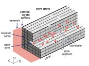
Fig.2: Model of a Zn(tbip) crystal as derived from the experimental findings and used in the Monte Carlo simulations.
