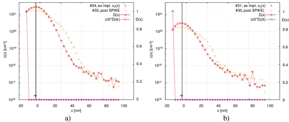
Figure 5: LDD model simulation test with parameter condition  $x_p=16$  nm and  $x_i$  minimal ( $\leq 4$  nm, depending on measured profile resolution) and the convolution approach in Equ. 1 for a) high dose ( $5 \times 10^{15} \text{ cm}^{-2}$ ) and b) low dose ( $5 \times 10^{14} \text{ cm}^{-2}$ ) Arsenic implant profiles  $c_0(x)$  (pls. compare Fig. 4a,c). Under this condition the initial Arsenic profile  $c_0(x)$  is approximated by the LDD model perfectly
