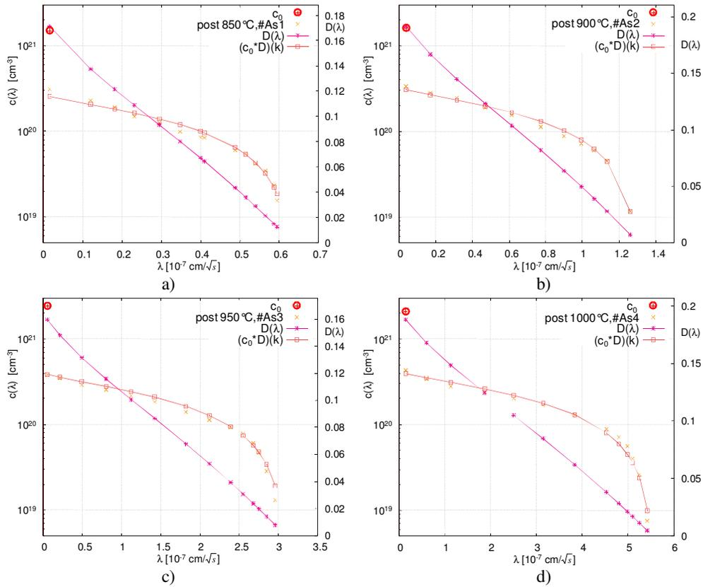
Figure 3: Arsenic SIMS profiles after surface diffusion experiments as published in Ref. [1] and LDD model approximation (“ $c_0^*D(k)$ ”, Equ. 7) by convolution approach as given in Equ. 1. Sample data and approximation parameters are listed in Tab. 2
