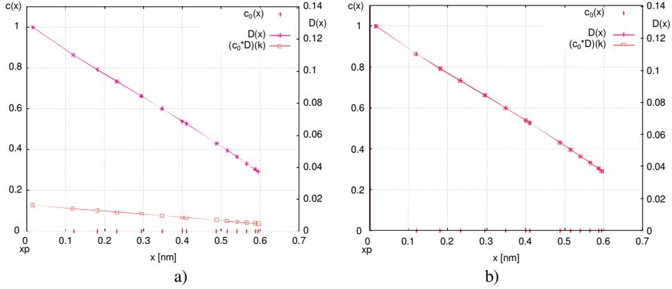
Figure 1: Mathematical convolution result of delta function like  $c_0(x)$  profile according to Equ. 2 with diffusivity function  $D(x)$  (Equ. 6) of LDD model for a)  $c_0=1$  and b)  $c_0=5.45$  according to Equ. 6 ( $D(0)=0.1835$ , see Equ. 4).
