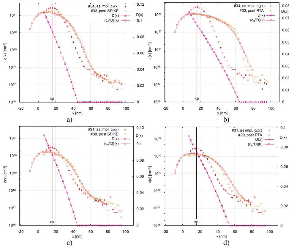
Figure 4: Arsenic SIMS spectra post implant and diffusion  $c(x)$  of samples #29-#34 (simulation parameters are given in Tab. 3), shown together with LDD model approximations by the convolution approach “ $(c_0*D)(k)$ ” as given in Equ. 1 (initial implant profile  $c_0(x)$ ,  $D(x)$  is LDD model’s diffusivity function).
