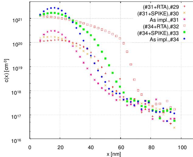
Figure 2: Arsenic SIMS profiles obtained from samples processed as listed in Tab. 1.
