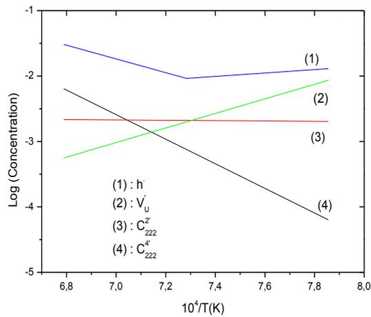
**Fig. 4:** Evolution of the various defect concentrations as a function of temperature, at  $P_{O_2}=10^{-10}$  atm.
