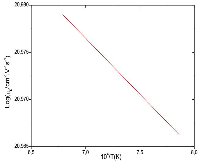
**Fig. 3:** Evolution of the electronic carrier mobility as a function of T.
