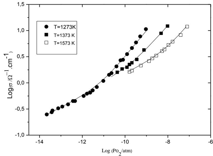
**Fig.1:** Adjustment procedure theory/experimental results of  $\sigma = f(P_{O_2})$  obtained by [15], for three temperatures.
