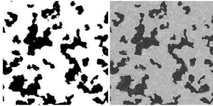
Fig. 2. Segmented (binarized) image. Pores are black. The raw image merged with interface of phases (white curves, right).
