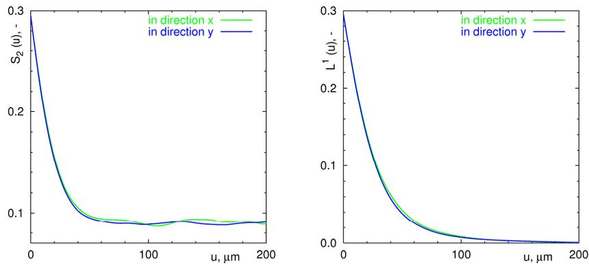
Fig. 3. Macroporous material C. Two-point probability function for the void phase (left), lineal-path function for the void phase (right), both in the principal directions.
