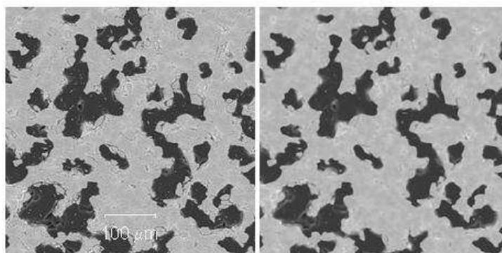
Fig. 1. Raw image of porous material C (left). Solid and void phases are respectively light and dark grey. Spatial filtration of the raw image using an adaptive median filter (right).
