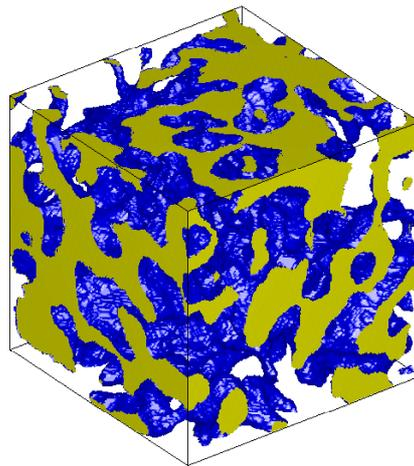
Fig. 4. 3D stochastic replica shown as a subregion of  $160 \times 160 \times 160$  voxels. Pore orifices are yellow, pore-solid interface is blue, and solid matrix is transparent.
