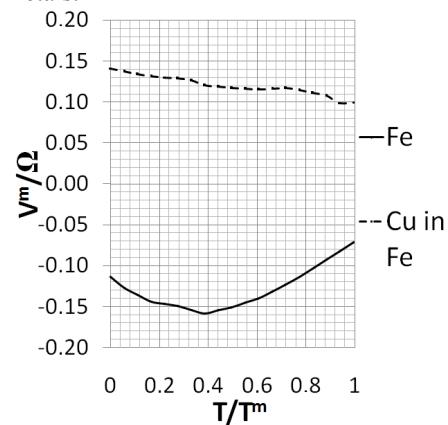
Fig. 1: Vacancy migration volume in BCC iron and migration volume for copper impurity atom jump versus temperature.
