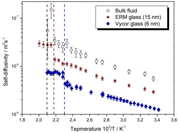
Fig. 1: Arrhenius plot of the bulk (open circles) and pore fluid (solid symbols) diffusivities for *n*-pentane in Vycor porous glass (diamonds) and ERM (stars) as a function of temperature. The vertical dashed lines show the positions of the bulk (black line) and pore critical points for Vycor (brown) and ERM (blue).
