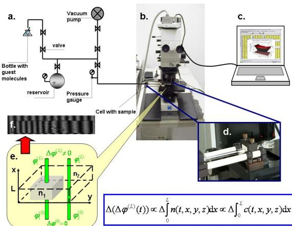
Figure 1: Schematics of diffusion measurement by interference microscopy (DIF)
