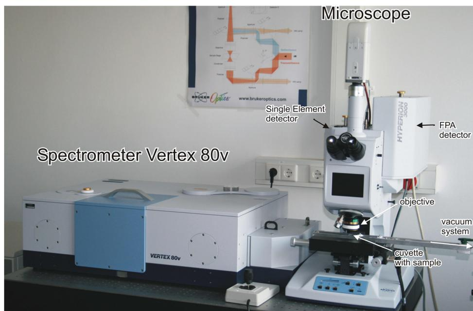
**Fig. 2:** IR micro-imaging device Bruker Hyperion 3000, consisting of a spectrometer and the microscope, with optics and detectors. The main part of the spectrometer is a Michelson interferometer.
