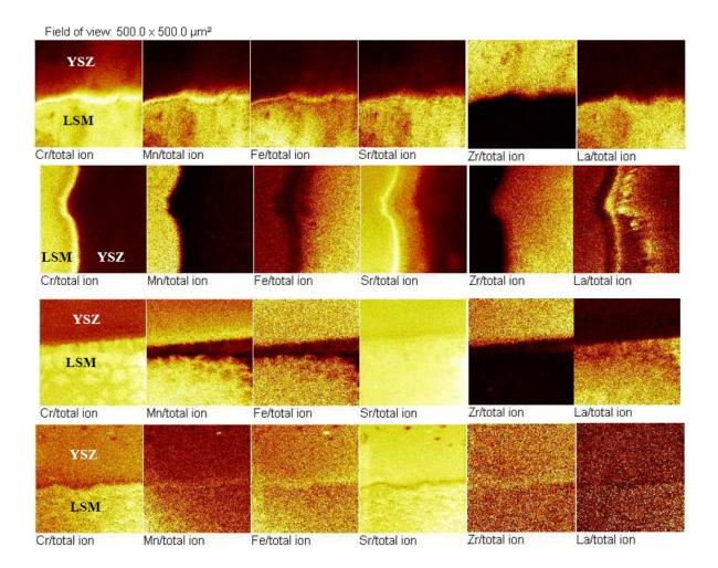
**Fig. 1** ToF-SIMS images of an LSM electrode on a YSZ sample. The whole sample was split into four smaller samples. Each quarter was annealed for different times at 1000 °C. The first line shows the sample as prepared without annealing. The other lines show the annealed quarters after 10 hours, 30 hours and 100 hours. Electrochemical polarization was not performed [3].
