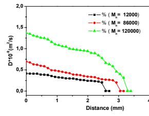
Fig.3. The diffusion profiles within the gel layer of HPMC taken along radial direction
