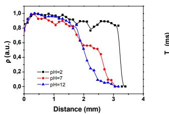
Fig.1. The spin-density  $\rho$  profiles of solvent protons within the gel layer of HPMC
