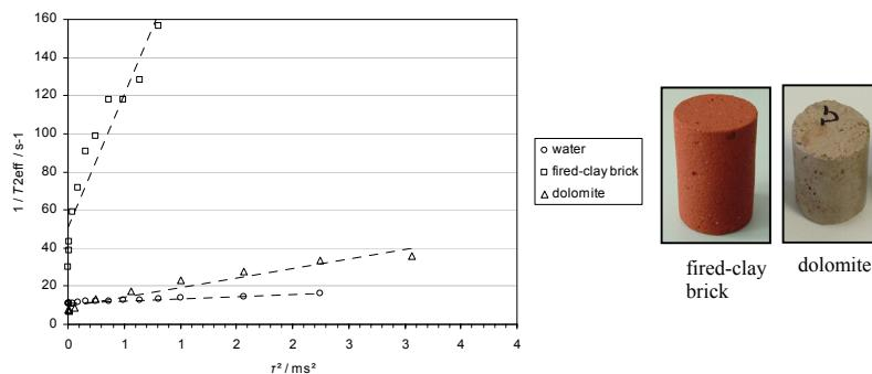
Fig. 1. Plot of the transverse relaxation rate against the echo time squared for a series of CPMG measurements using a low-field NMR spectrometer (9.1 MHz). Samples are bulk water, a water-saturated fired-clay brick and a dolomite rock (photographs).
