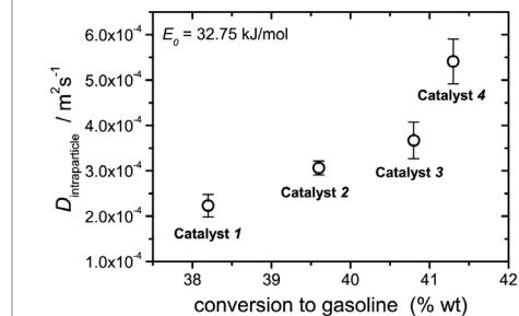
Fig.3 Correlation between the intraparticle diffusivity of n-octane and catalytic performance expressed by the oil-to-gasoline conversion for the same catalyst-to-oil ratios.
