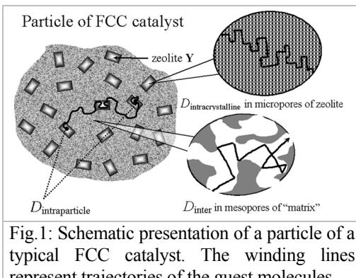
Fig.1: Schematic presentation of a particle of a typical FCC catalyst. The winding lines represent trajectories of the guest molecules.
