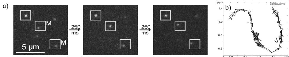
**Fig. 1:** a) Sequence of images acquired with the wide-field imaging setup (14 ms per frame; 17 frames (ca. 250 ms) are skipped between the depicted images). The fluorescence patterns of 1 immobile (I) and 2 mobile (M) molecules are highlighted. b) Structured trajectories occur in the case of a well-ordered system of channels like hexagonal SBA-15.
