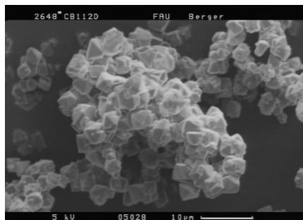
**Figure 1:** Crystals of zeolite Y obtained without ageing.
