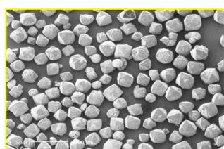
Fig. 1 : SEM micrograph of the NaX sample
