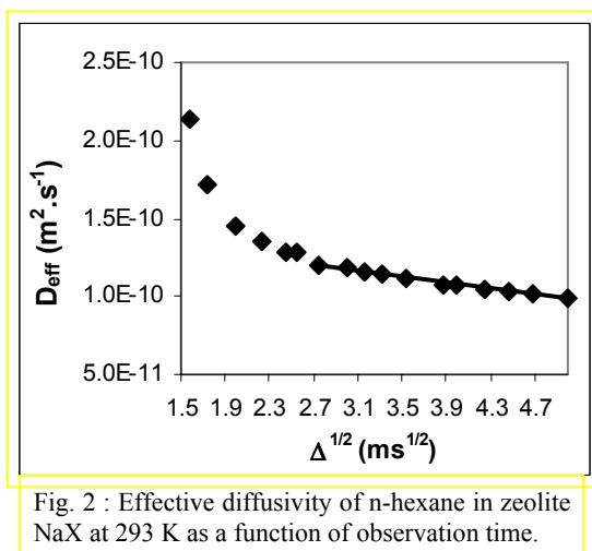
Fig. 2 : Effective diffusivity of n-hexane in zeolite NaX at 293 K as a function of observation time.
