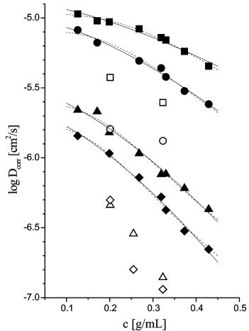
Fig.1: Dependence of the diffusion coefficients of the tracers on the polymer concentration in solutions of poly(HEMA) (■ IV, ● V, ▲ VIa, ◆ VIIb) and in HEMA gels (empty symbols).
