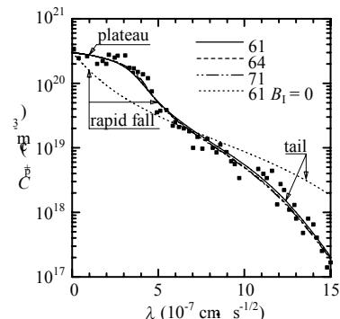
Fig. 1: Experimental P diffusion profile and its simulation. [1,3]
