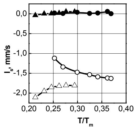
Fig. 1.  $I_s$  temperature dependences of components 1 ( $\bullet, \blacktriangle$ ) and 2 ( $\circ, \triangle$ ) in  $^{119m}\text{Sn}$  spectra of PC ( $\bullet, \circ$ ) and NC Nb ( $\blacktriangle, \triangle$ )
