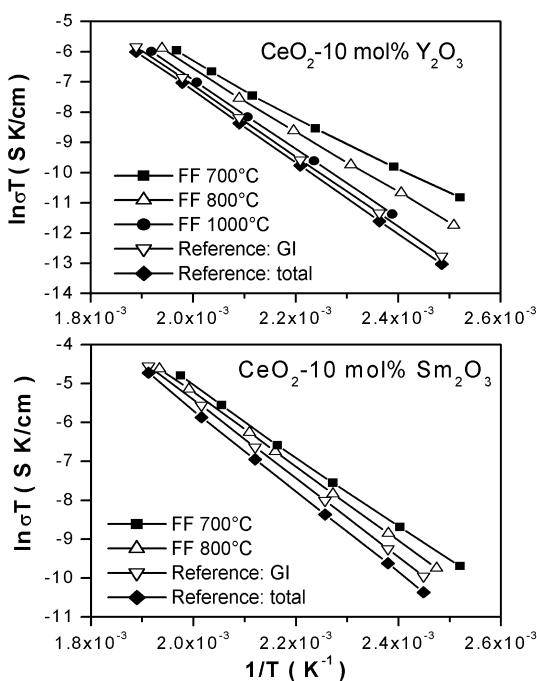
**Figures 1a and b:** Arrhenius plots:  $\text{CeO}_2\text{-}10 \text{ mol\% Y}_2\text{O}_3$  and  $\text{CeO}_2\text{-}10 \text{ mol\% Sm}_2\text{O}_3$  ceramics, for different grain sizes.
