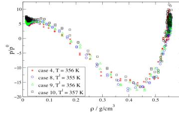
Fig. 1: Pressure parallel to the surface as a function of the local density in the surface, at equilibrium (case 4) and out of equilibrium (cases 8, 9 and 10), the cases mentioned referred to the situation of ref [4]. The calculated heat fluxes equaled, respectively, 27.0, 41.3 and 69.0 MW/m<sup>2</sup>, for the cases 8, 9 and 10.
