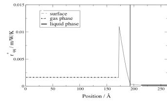
Fig. 2: Profile of the thermal resistivity across the surface for state 7 of ref [4], (the heat flux equal  $23.9 \text{ MW/m}^2$ ). The values of the liquid and gas phases are shown as constants. The position of the equimolar surface is shown by a vertical line.
