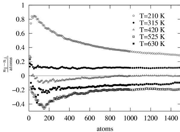
**Fig. 1** Anisotropy parameter  $n_{||} - n_{\perp}$  as a function of the size of a growing cluster averaged over 10 realizations of the growth process. The mean sampling error at 1000 atoms is about  $\pm 0.03$ . The simulation also includes exchange processes (see text) with an activation barrier twice as high as the diffusion barrier.
