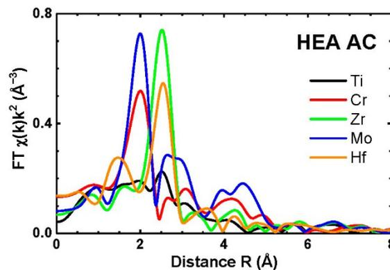
**Fig. 3.** Comparison of the Fourier transform of the EXAFS spectra for as-cast (AC) TiZrHfMoCr HEA at the K-edges of Ti, Cr, Zr, and Mo and L<sub>3</sub>-edge of Hf. Only the moduli of FTs are shown for clarity. Reprinted with permission from Ref. [1]. Copyright 2023 MDPI.
