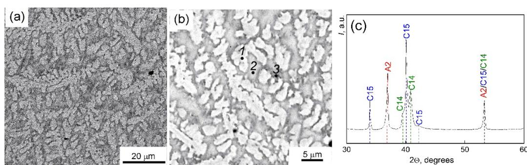
**Fig. 1.** SEM images of the initial microstructure of the TiZrHfMoCr alloy: (a) general view, (b) dots mark the areas of component analysis: light gray (1), dark gray (2), and gray (3) colors. (c) X-ray diffraction pattern of the as-cast TiZrHfMoCr alloy. Reprinted with permission from Ref. [1]. Copyright 2023 MDPI.
