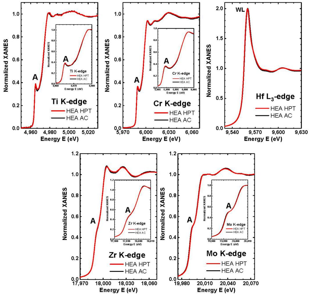
**Fig. 2.** XANES spectra of the original as-cast (AC) TiZrHfMoCr HEA sample and sample after HPT at the Ti, Cr, Zr, and Mo K-edges and Hf L<sub>3</sub>-edge. The insets show an enlarged view around the edge. The pre-edge A and the white line WL are indicated. Reprinted with permission from Ref. [1]. Copyright 2023 MDPI.
