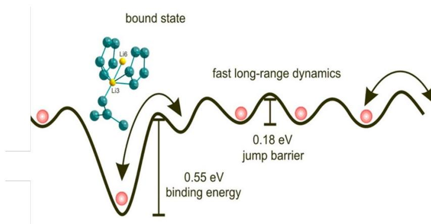
**Fig. 1.** Sketch of the energy surface of Li (red) in the lithium silicide  $\text{Li}_{12}\text{Si}_7$ . Long-range diffusion is characterized by a hopping barrier of 0.18 eV. Additionally, there are bound states—sites on which Li is bound more tightly. The long-range process is not interrupted by the bound states (here, it only appears so owing to the 1D projection). Adapted from [4] with permission.
