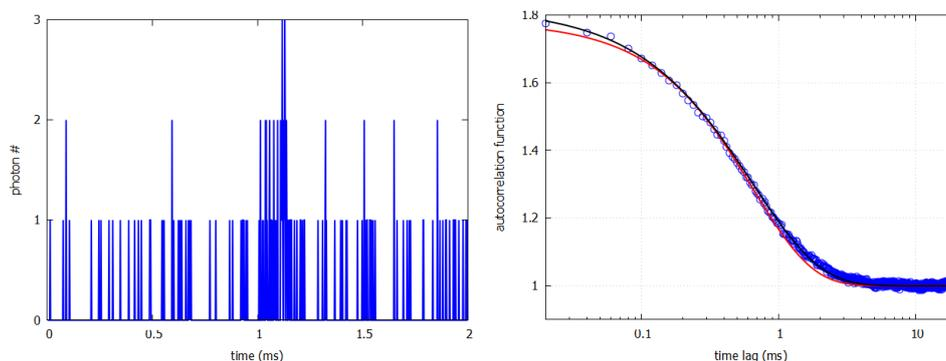
**Figure 1:** Left: sketch of photon bunches scattered by fat particles in milk. Right: autocorrelation function calculated from light scattering on milk as a function of time lag between scattering events. Red line is a simple exponential fit, black line is fitted with a normal distribution of particle diameters.
