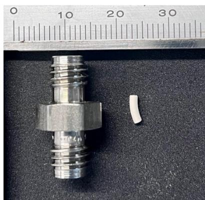
Figure 1: Zero Length Column and 5A commercial pellet used in the experiments.
