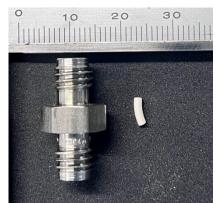
Figure 1: Zero Length Column and 5A commercial pellet used in the experiments.
