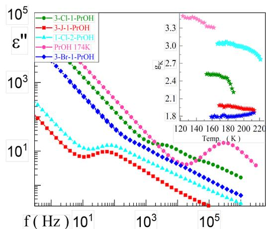
Figure 1: Imaginary part of dielectric complex permittivity frequency-dependent  $\epsilon''(f)$  at 173 K. Inset shows Kirkwood-Fröhlich factor of the studied alcohols.
