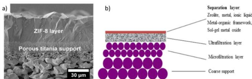
a) A metal-organic framework (MOF) type ZIF-8 layer on an asymmetric graded titania support [4], b) Principle of a supported membrane: The  $\mu\text{m}$ -thick separation layer is deposited on a
