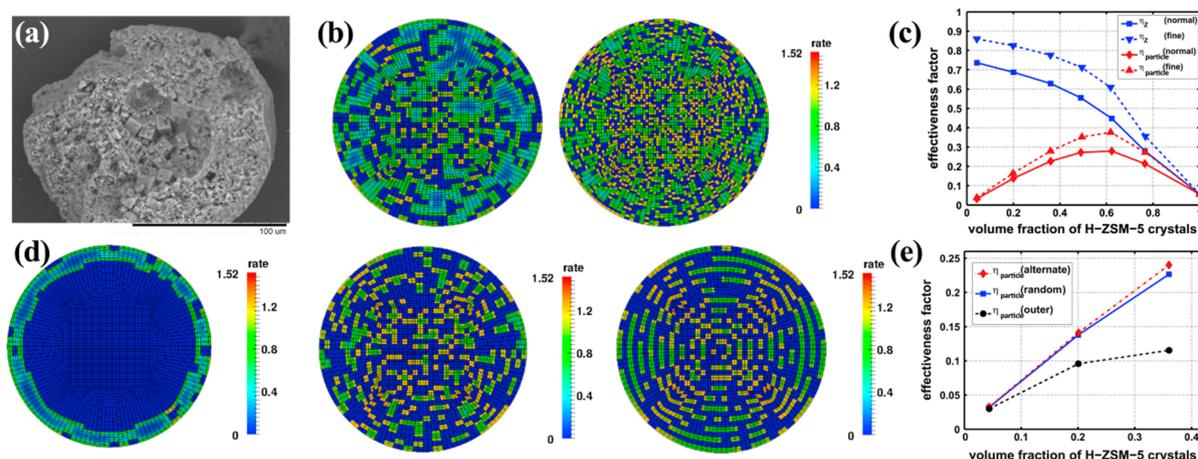
Figure 1: (a) Interior of catalyst particle used in industrial process. (b) The distribution of zeolite and reaction rate inside catalyst particle with volume fraction of H-ZSM-5 of 0.62. (c) Effectiveness factor as a function of volume fraction of H-ZSM-5 for both normal and fine crystal sizes. (d) The spatial distribution of zeolites and reaction rate inside catalyst particle. (e) Effectiveness factor for zeolites with different spatial distribution.
